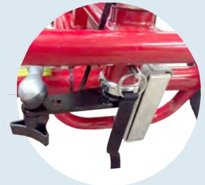
PLUS Rear Steering Kits on all trykes can be converted to a push bar by inserting a pin.
