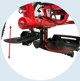
Upgraded foot platforms adjust independently up/down, right/left, tip heel or toe up/down.
