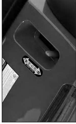
5 Freewheel Function Manual driving without batteries
