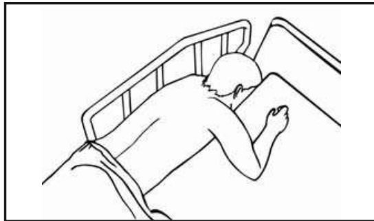
Zone 3 – Entrapment between the rail and the mattress
