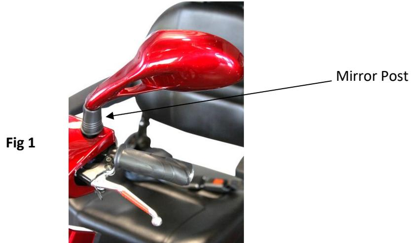
To attach the mirrors simply place each mirror threaded end into the mirror post. Turn mirror clockwise and fasten mirror to scooter.
