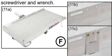
**Step 12.** If you are displaying your license plate on the carrier, use the License Hanger (10). Pull the pin on the front of the Hanger and slide the tab on the back of the Hanger into the top slot of the Adapter. Let go of the pin and it will lock place. If you are just using a light on the carrier, install the Light Hanger (11) instead of the License Hanger.
