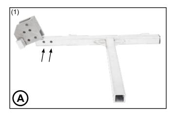
**Step 2.** Apply two 15/16" bolts (7) with a washer on each side of the Connection Block followed by the lock washer and then the nut for each bolt. Securely tighten both bolts with wrenches. Proper tightness will help keep the carrier quiet during use. See page 7 for details about attaching the Bogie Wheel (sold separately).
