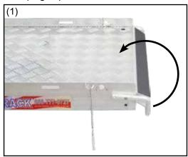
**Step 2.** Align the small hole in the end bar to the small hole in the carrier unit frame.
