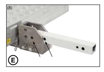
**Step 9.** The Hitch Bar should fit snugly so that your carrier is quiet. Install the last 15/16" bolt with a washer on each side, lock washer, and nut as previously done in Step 2. Tighten the bolt with a wrench and/or socket wrench.
