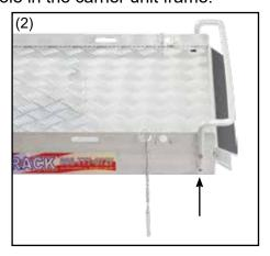
**Step 3.** Using the pins attached to the chain, insert one into the hole on each side of the carrier. Please note that this is a tight fit. To release the end bar, simply remove the pins and rotate the end bar down.
