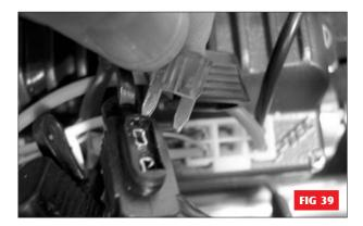
For access to a fuse remove the four screws located in the rear body cover, lift cover. Locate and lift the fuse block on it's wire, lift up the fuse lid and withdraw the 'read' fuse. Replace the blown fuse with recommended 10amp (pink) fuse, close fuse lid and replace fuse block.
