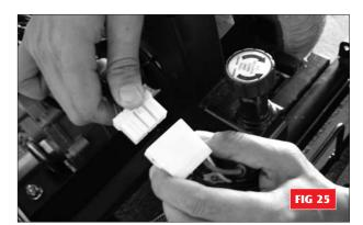
can only be reconnected together one way. Note the locating lugs on the connectors, do not force these connectors together when refitting.
