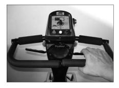
**DELTA CONTROLLER** For Scooter users with limited hand dexterity. Allows the user to control the Scooter by pulling the lever toward themselves.
