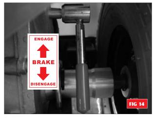
**General Note:** If you are able to push your scooter the drive to the transmission brake is disconnected. Do not attempt to drive your scooter. Please check once more the above mentioned procedure for re-engaging the drive.
