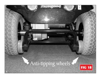
**PLEASE NOTE:** The rear stability of your Scooter is dependent on a number of factors which you should consider before attempting to climb an incline or other obstacle: (a) your height; (b) the height of your seat; (c) your weight and (d) the angle of the incline you are attempting to climb. All of these factors can affect the rear stability of your **Freerider** Scooter. If you are unsure of your capability to climb an obstacle, then try another route - always think 'safety first'.
