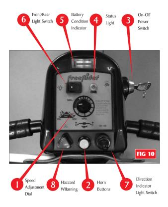
diagnostic system which can identify faults which could occur on the main speed control system or some other part of your Scooter's electronic drive system. For instance if your batteries run low in power, the status light will flash slowly at one flash a second; this indicates your batteries need recharging.
