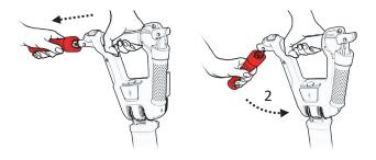
21. Hold the console, on the bottom of the tiller open the lever, push the tiller gently down. close the lever.
