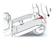
left hand push down the front handle (red in the illustration below) to lock it in position (make sure to do that when the tiller is vertical).
