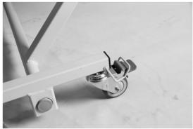
3. To unlock the casters, step on the "Off" lever at the rear of the bed. Lift up the caster guides on the head end casters to allow free movement.
