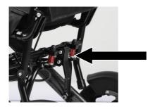
Step 2: Hold the handlebar with one hand and the seat cushion frame with the other. Use both hands to force the wheelchair until it is completely folded.
