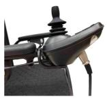
When the indicator light of the charger turns green, unplug the plug of the charger, then pull out the power plug.
