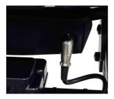
5: Pull up the Both Motor clutch fork, keep them on electric operation state. The wheelchair cannot be pushed by hand, and this will prevent the wheels from rolling.
