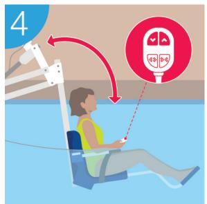
Lower lift into the water using the down button.
