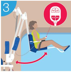
Rotate the lift above the pool using the appropriate buttons.
