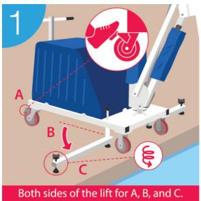
Position the lift. Lock rear casters (A), deploy outriggers (B), and twist pressure foot on both sides all the way to the ground (C).
