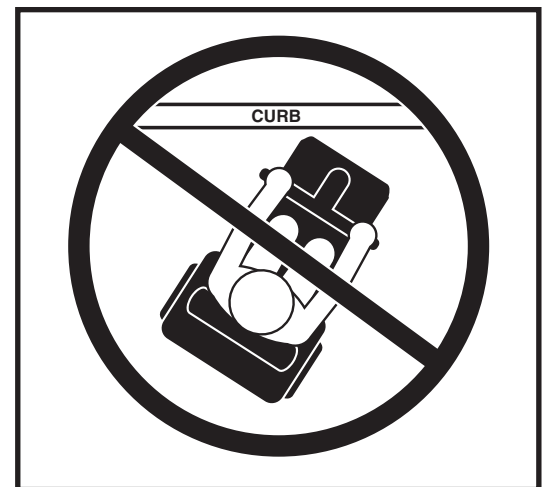
Figure 7. Incorrect Curb Approach
