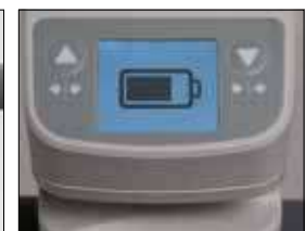
Battery charge indicator on hand pendant and LCD Display
