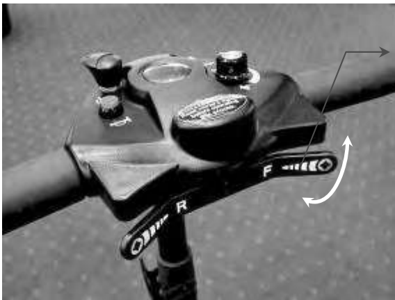
Finger Lever Control/Maximum Force Applied on Lever is 4N
