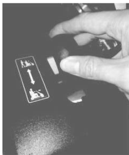
Disengage and in freewheel mode.
