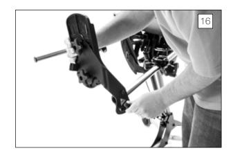
17. If the hip supports were ordered, insert hip supports into the bracket behind the pelvic pad. Tighten securely.
