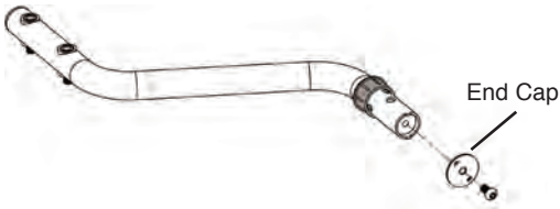
FIG. 10- On the support arm, remove the plastic bag with two mounting bolts and a silver pin. Using a hex wrench, remove the end cap from the Shadow Tray arm.
