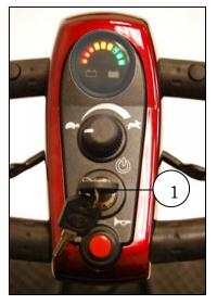
Figure 12. Key Switch (On)
