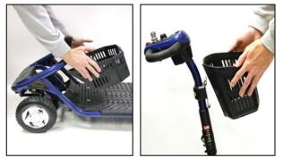
Figure 15. Removing the Baskets
