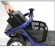
Figure 21. Battery Pack Installation
