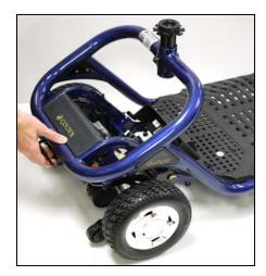
Figure 17. Releasing the Drivetrain
