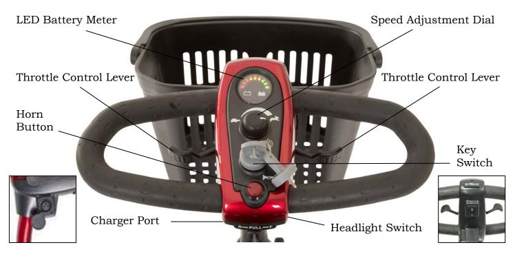
Figure 5. LiteRider<sup>™</sup> Delta Tiller Control Panel
