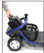
Figure 13. Removing the Seat
