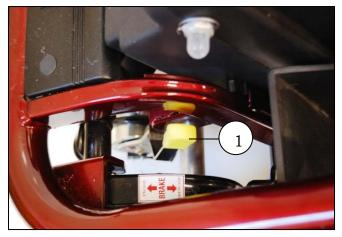
Figure 9. Freewheel Mode (Brake Disengaged)
