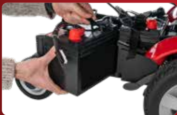
Side access to the battery
