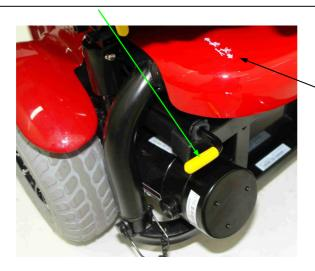
Sticker indicating position the brakes are locked or unlocked.
