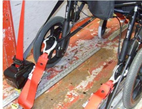
Fitting the rear restraint
