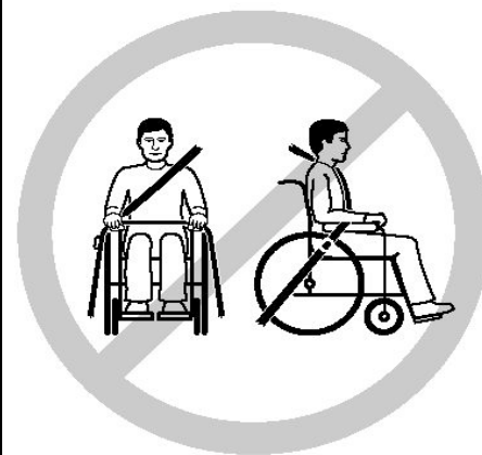
Incorrect seat belt position
