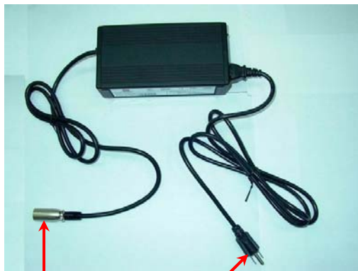
plug-in controller plug-in wall outlet
