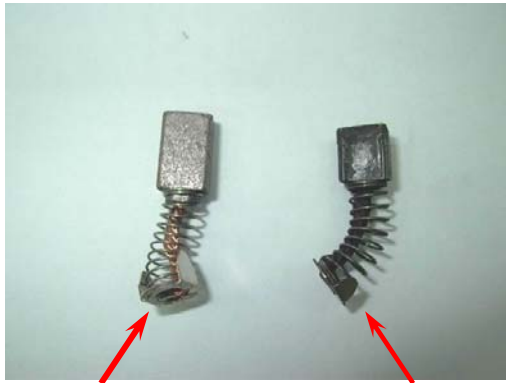
New Motor Brush Worn Motor Brush (Fig 17)
