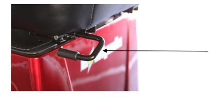
2. Locate the reclining seat lever located on side of seat.
